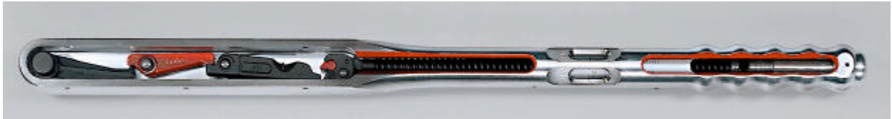
Figure 4. Multi-lever inside mechanism of a clicker torque wrench.
